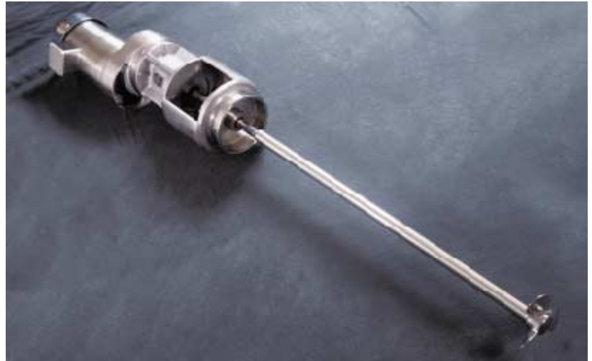
(Above) Electropolished and passivated stainless steel castings and fabrications make up the mixer drives on SHARPE's all stainless steel series mixers. Shown here is a 350 RPM unit with a sanitary ferrule mount and mechanical seal.
