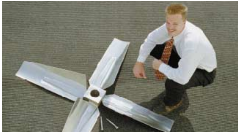
Impellers are available in various configurations from simple propellers to complex helix designs. Split impellers (shown above) with teflon gasketed assembly points allow ease of installation and adjustment while providing easy-clean characteristics. For more stringent polishing needs, the impellers are welded to the shafts and all welds blended and polished.
