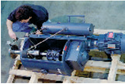
(Above) Shaft runout is checked on an N-Series UNIMECH™ drive.
