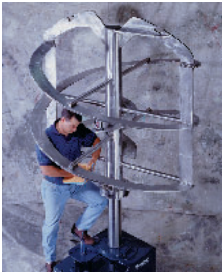
(Below) A double flight helix/anchor impeller is one of many designs we build for more viscous products.
